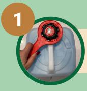
While the drum is upright - remove black top lid. Bung Tool makes removing easier.
