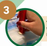
While the drum is upright - remove black top lid. Bung Tool makes removing easier.
